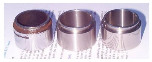
The piston on the left came from the rear end of Kirby Palm's '83. That's not dirt; that's all rust, including the line part way around the side on the sealing surface. The OEM pistons are chrome-plated steel, and eventually the steel rusts and the chrome plating flakes off. This one survived 17 years so one cannot fault their durability, but when they start to look like this they tend to cause pesky problems like sudden brake failure.
