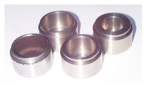
The one at the front left is one that came out of the car. Rust galore. The faint lines on the sealing outer surface are not dirt; that's where the chrome plating has begun to crack and rust is starting to break through.
